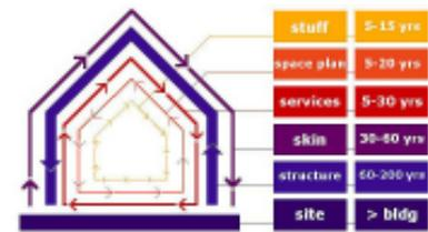
Left, each “layer” of a building has a different life span (after Stewart Brand, 1994)
